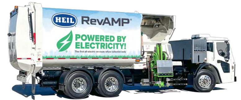
EV Automated Side Loaders
